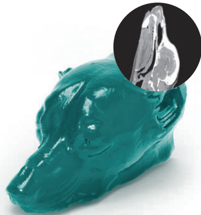
Dog's head Phantom for CT and X-ray
